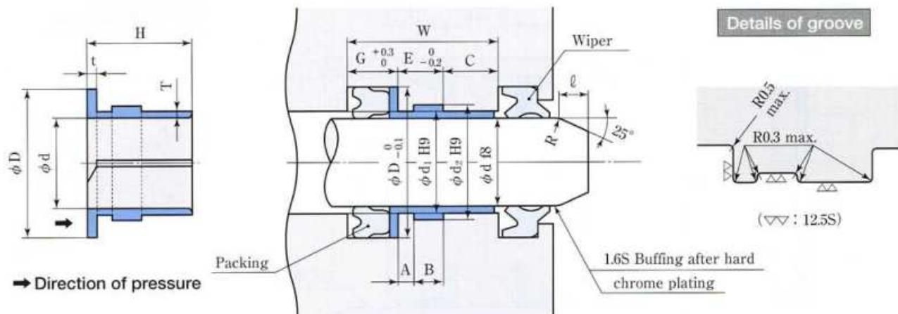
Note: ● S-LLEEVE® should be installed in the direction specified on the above schematic.
