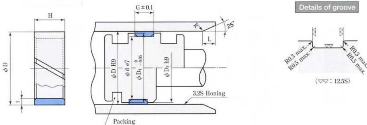
Note: ● Refer to the L dimension as it would be differed according to the type of packings to be used together.
