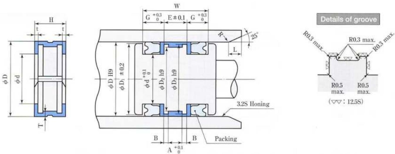
Note: ● Refer to the L dimension as it would be differed according to the type of packings to be used together.
