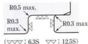
Note: ● Adopt divided grooves. However, note that D=140 for pistons and larger sizes, and d=80 for rods and larger sizes are installable in one-piece groove. In these cases, specify back-up rings with bias cut (TC-KY-○○).
