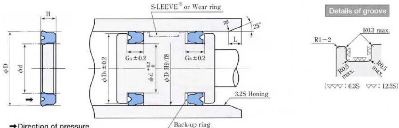
Note: ● Packings should be installed in the direction specified on the above schematic.
