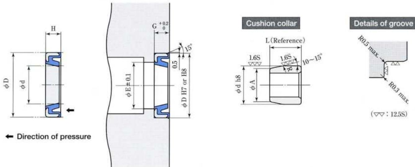
Note: ● Cushion seals should be installed in the direction specified in the left schematic.
