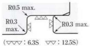
Note: ● Adopt divided grooves. However, note that D=140 for pistons and larger sizes, and d=80 for rods and larger sizes are installable in one-piece groove. In these cases, specify back-up rings with bias cut (TC-KY-○○).
