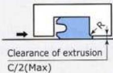
Fig. C Combination with back-up rings
