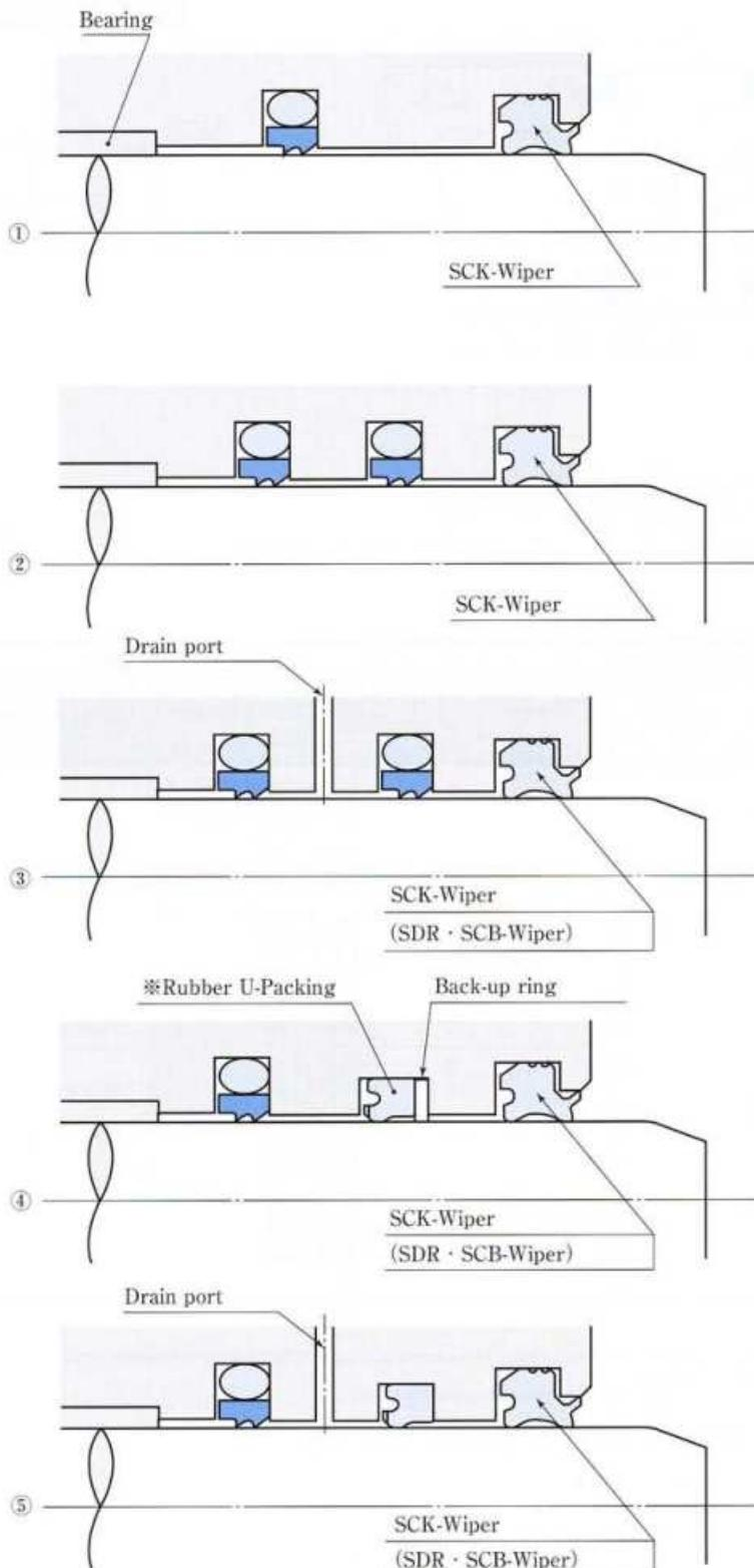
① This is an example of the sealing for a basic cylinder. Although it has small leakage, the emission of the pressure oil from the outer side of the wiper avoids the damage caused due to the extrusion and the breakage.
