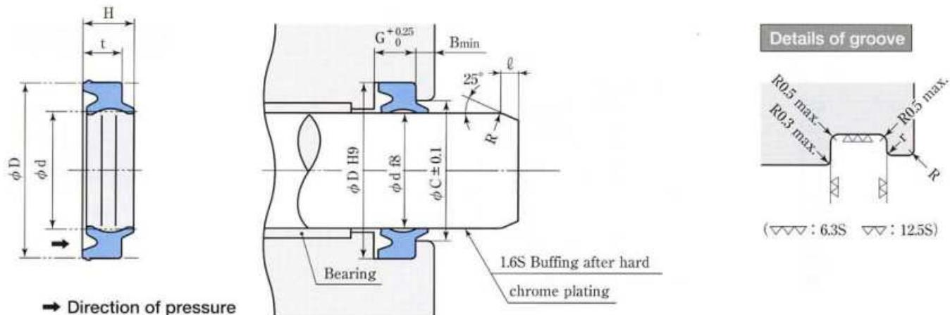
Note: ● Packings should be installed in the direction specified on the above schematic.
