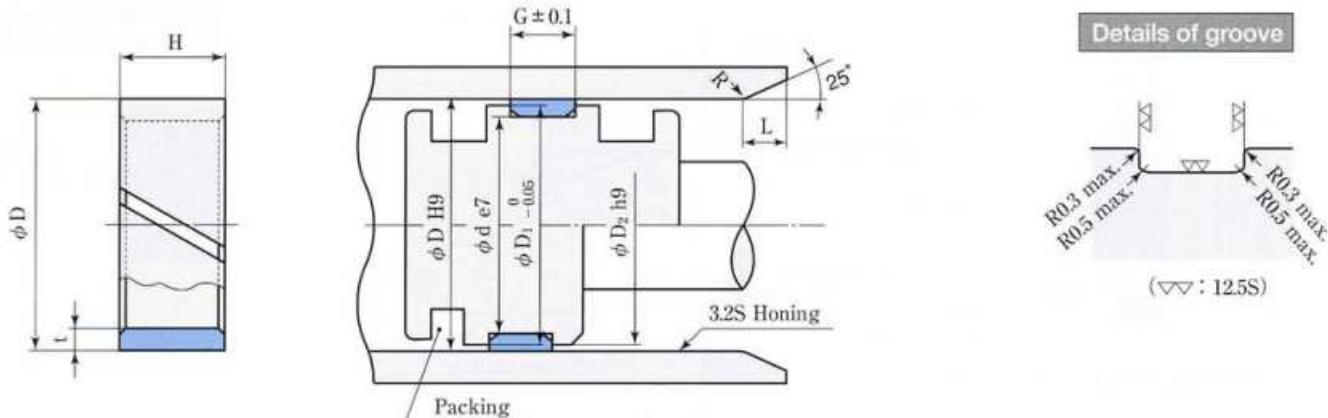
Note: ● Refer to the L dimension as it would be differed according to the type of packings to be used together.
