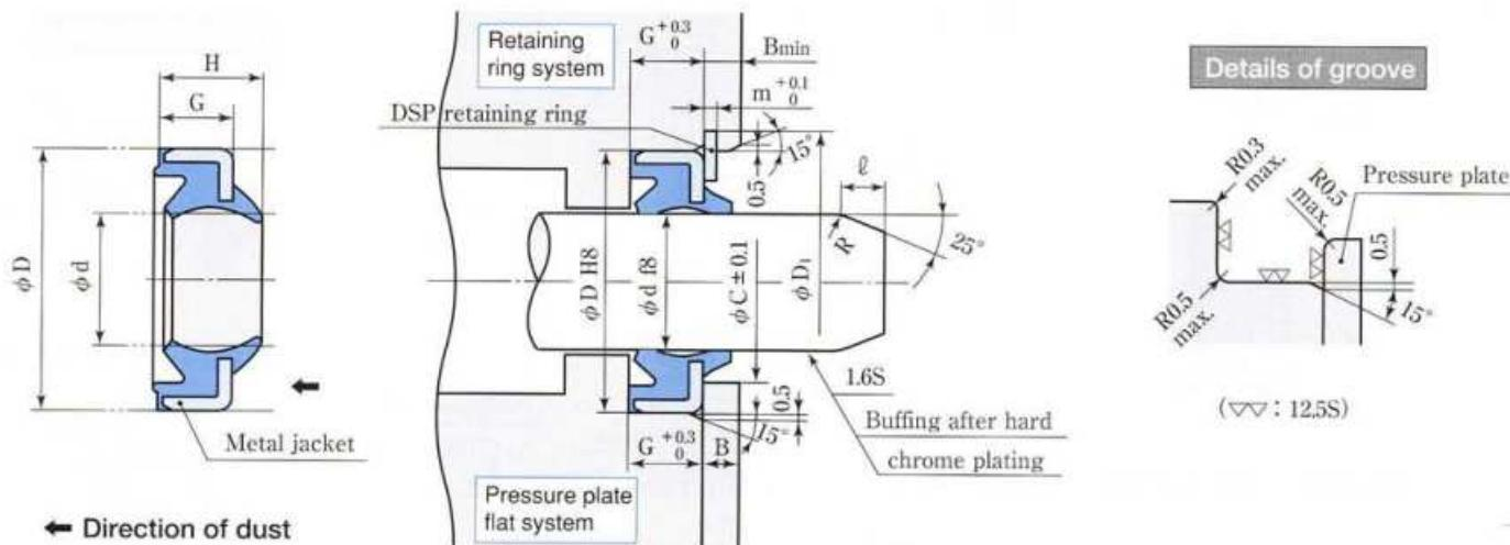
Note: ● Wipers should be installed in the direction specified in the above schematic.
